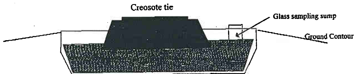
Figure 1. Schematic diagram illustrating the mesocosm layout for a study to examine PAH migration from creosote treated railway ties.
